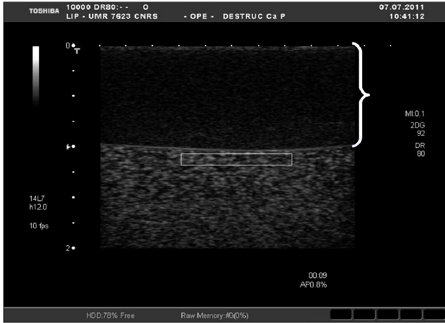
Figure 3.1: Image acquired during the dose ranging experiment ( 2 \times 10^5 microbubbles/mL). The bracket designates the gelatin stand-off placed between the transducer and the surface of the microbubble suspension. The white rectangle delimits the region of interest in the contrast agent suspension from which average echo-power was calculated. Image pixel values were converted into echo-power using custom software developed by our group [50].
